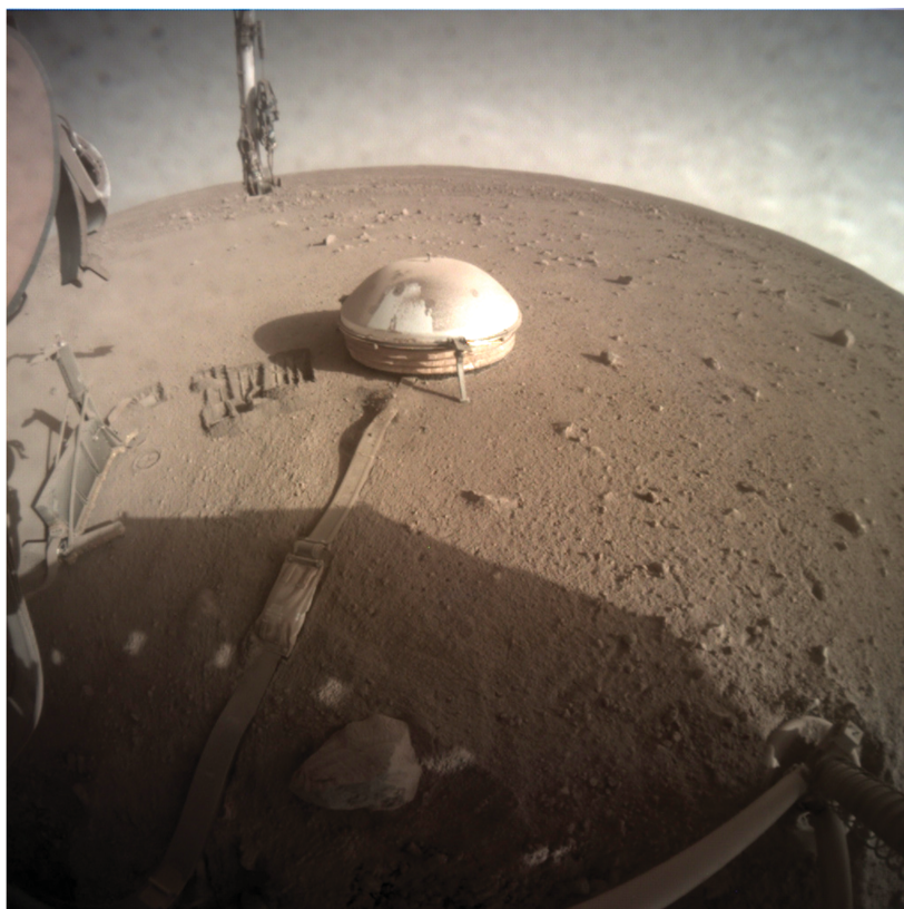
Figure 1. (a) The sensor assembly of the Seismic Experiment for Internal Structure of Mars (SEIS) on the ground just prior the deployment of the Wind and Thermal Shield (WTS), on 2 February 2019. (b) Picture taken on 27 September 2021 showing the fully installed WTS two and a half years later. These two images were taken on sol 66 and sol 1008 since InSight landing, respectively.
