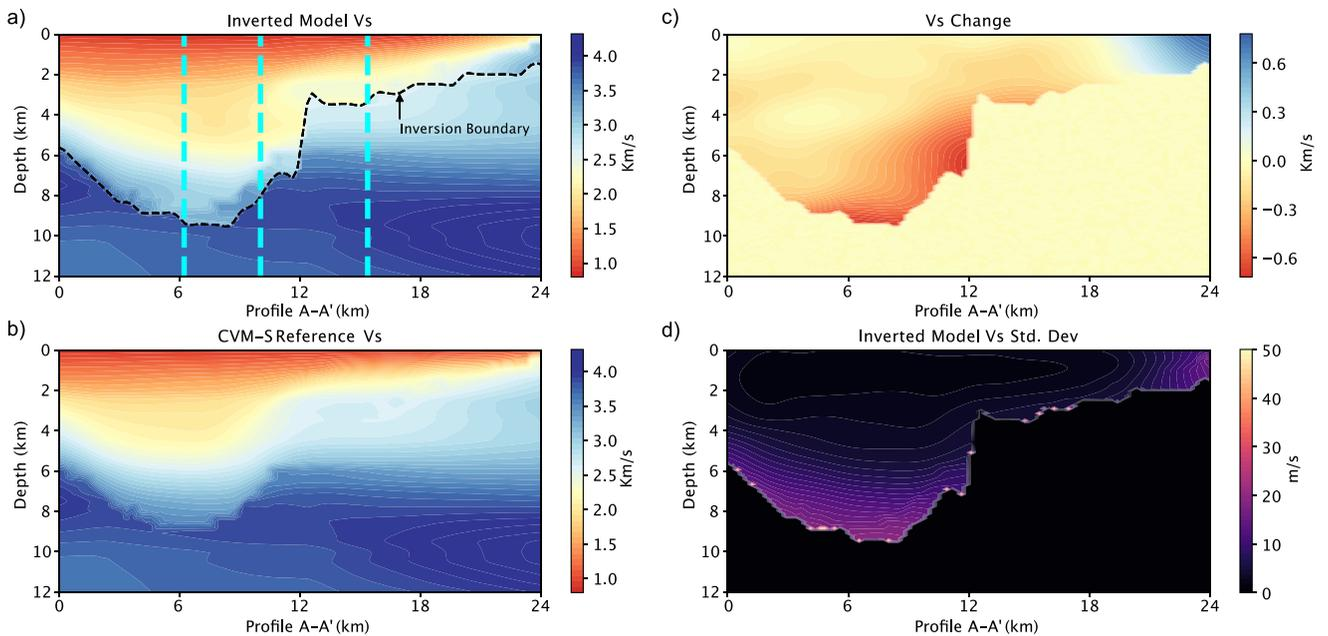
**Figure 12.** (a) Mean of the final ensemble  $V_s$  model, (b) CVM-S reference model  $V_s$ , (c) difference between final model and reference model, (d) standard deviation of the final ensemble  $V_s$  model.
