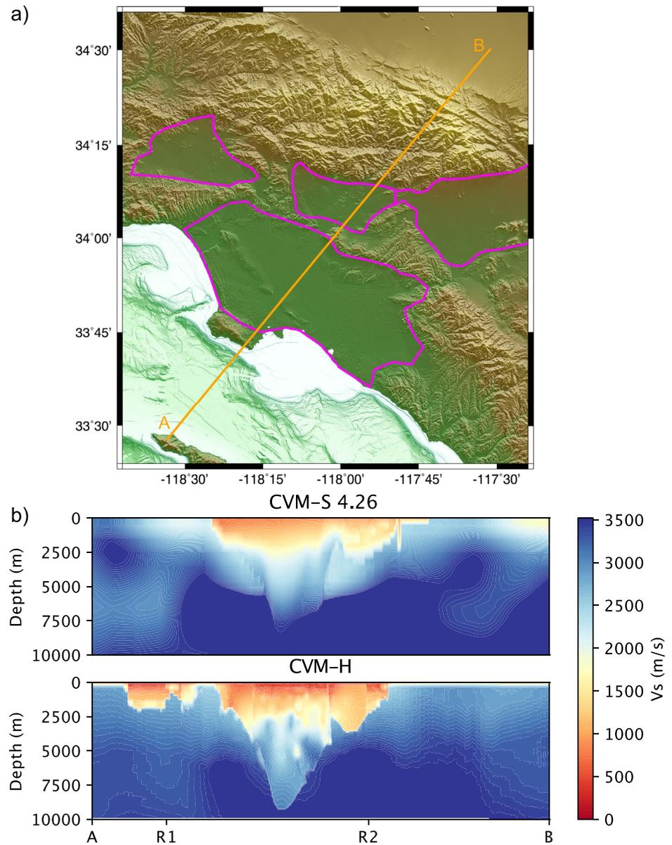
**Figure 1.** (a) Shaded elevation model of southern California showing the outline of the major basins (defined by slope-break analysis) in purple and the transect A-B used for profiles shown in orange. (b) Characteristic profiles through the Los Angeles basin for the CVM-S and CVM-H models. Abrupt lateral changes in resolution at positions R1 and R2 are seen in the CVM-H model.
