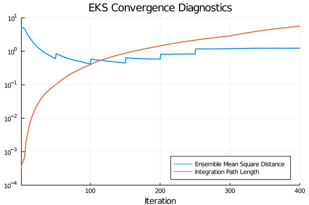
**Figure 10.** Convergence diagnostics of the Ensemble Kalman Sampler (EKS) showing the Mean Square Distance between ensemble members converging to a constant, which suggests the ensemble has reached an equilibrium and is approximating the posterior. The integration path length steadily increases, showing that the ensemble is not being forced to take very small steps (heuristics from Garbuno-Inigo et al. (2020) suggest a path length of 2 is sufficient to approximate the posterior).
