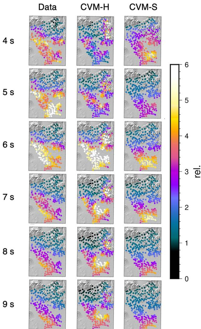
**Figure 3.** Relative amplification of the maximum amplitude of 3 component pseudo-spectral accelerations (PSA) in the range of 4–9 s from the Mw 7.1 5 July 2019 Ridgecrest earthquake as recorded on the Community Seismic Network (CSN), and as simulated using the Graves and Pitarka rupture generator (Pitarka et al., 2019) and a 3D finite-difference waveform solver for both the CVM-H and CVM-S models (Graves, 1996).
