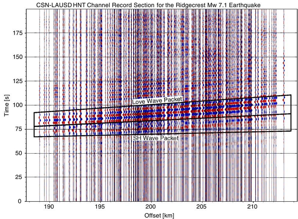
**Figure 4.** Record Section of the Mw 7.1 Ridgecrest earthquake as recorded on the HNT channel of the CSN-LAUDS array, zero-phase bandpass filtered between 4 and 10 s. Two main phases are clearly identifiable, with the first arriving phase exhibiting little delay due to the basin at longer offsets, which we infer to be the primary SH arrival. A second, stronger phase, which is delayed by the basin at longer offsets, we infer to be the fundamental Love mode.
