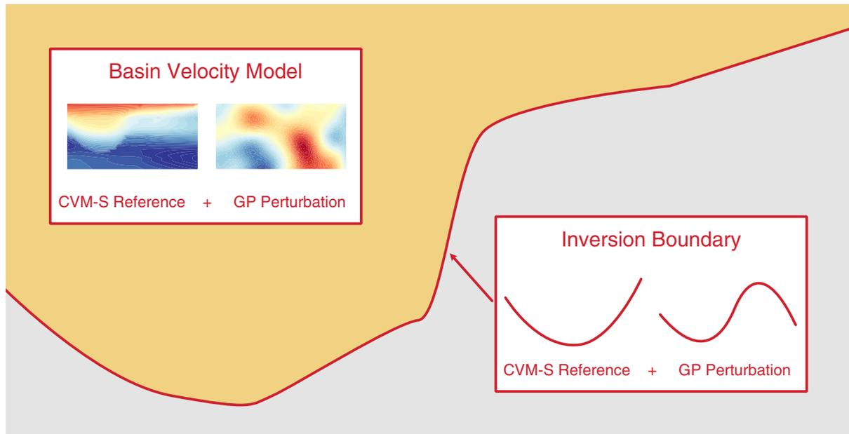
**Figure 7.** Schematic of the model definition, showing the construction of the velocity model update and the boundary of the inversion, both constructed from a CVM-S reference perturbed by a Gaussian Process. The background model, schematically shown in gray, is given by the unaltered CVM-S model.
